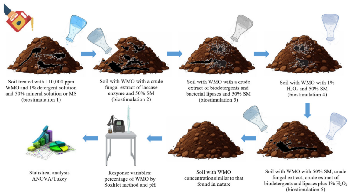
Figure 1. Diagram of biological recovery of an agricultural soil impacted by 110,000 ppm of waste motor oil
